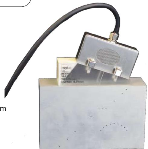
Probe with TPAC wedge and 85 mm thick aluminum SDH test piece
